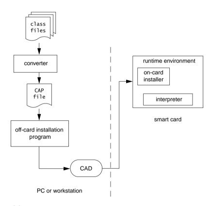
Figure 3.3 Java Card installer and off-card installation program
